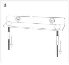
Pull the wire through the hole in the top fixing bracket so the threaded ball rests in the hole. Repeat the same steps with another wire at the other end of the top bracket
