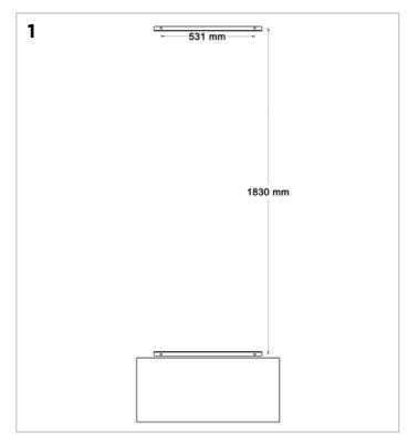
Mark out the position where the trellis will be attached to the wall. The hole centres in the brackets are 531mm and the hole centres vertically between brackets need to be 1830mm. Note: Overall dimensions of the trellis including brackets will be 605mm x 1850mm.
