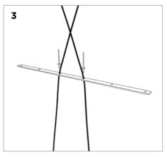
Cross the two wires over each other and feed the stud ends through the two inside holes on the spreader bar.
