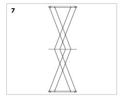
Repeat steps 1 to 6 for all wires working from the outside holes to the inside holes on the fixing brackets (inside to outside holes on the spreader bar). **IMPORTANT:** Follow the weaving pattern as per *figure 1*. on page 4.
