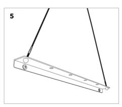
Attach the threaded balls to the stud ends through the bottom fixing bracket. Rotate the ball so the wires are tensioned enough to support the spreader bar.
