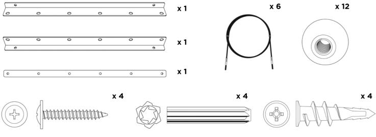
8g x 30mm Screw. Suitable for fixing into timber or using with plastic plugs. For maximum hold and where possible screws should be attached directly to wall studs. 6mm x 30mm Red wall plug. Suitable for fixing into concrete, stone, solid brick and solid block. Wall plugs suit a 6mm pre-drilled hole. Nylon Plaster Board Anchor. Suitable for fixing into plaster board. Install using a power drill and Phillips drive bit.
