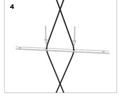
Cross the wires back over each other before attaching to bottom bracket. **IMPORTANT:** Follow the weaving pattern as per *figure 1*. on page 4.
