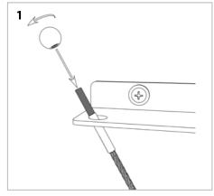
Feed the stud on the end of a wire through the outside hole on the top bracket. Attach the threaded ball onto the stud. Rotate the ball 2-3 times so it holds on the stud.
