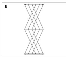
Tension all the wires top and bottom so they are firm but not tight. **Caution:** Over tensioning the wires may cause the fixing brackets to sag and may put extra stress on the fixing screws.
