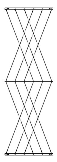
It is recomended to follow the weave pattern as shown above. Wires should be weaved over-under-over-under and so on. Following this pattern will ensure the trellis does not twist. A wire that is weaved over the last wire above the spreader bar should be weaved under the first wire below the spreader bar. A wire that is weaved under the last wire above the spreader bar should be weaved over the first wire below the spreader bar.
