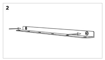
Attach the top bracket to the wall. **Note:** the the screw holes in the bracket should be at the top. The bracket should be level when attached to the wall.
