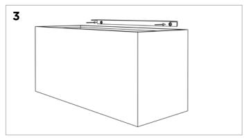
Attach the bottom bracket to the wall. **Note:** the screw holes in the bracket should be at the bottom. It is recomended to have a small gap (at least 10mm) between the bottom of the bracket and the top of the planter box.
