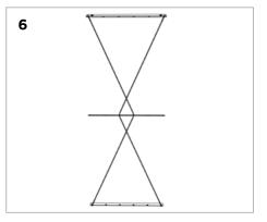
Level the spreader bar and position in the middle between the top and bottom fixing bracket.
