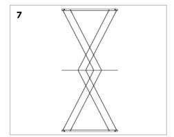
Repeat steps 1 to 6 for all wires working from the outside holes to the inside holes on the fixing brackets (inside to outside holes on the spreader bar). **IMPORTANT:** Follow the weaving pattern as per *figure 1*. on page 4.
