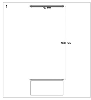
Mark out the position where the trellis will be attached to the wall. The hole centres in the brackets are 763mm and the hole centres vertically between brackets need to be 1830mm. Note: Overall dimensions of the trellis including brackets will be 840mm x 1850mm.
