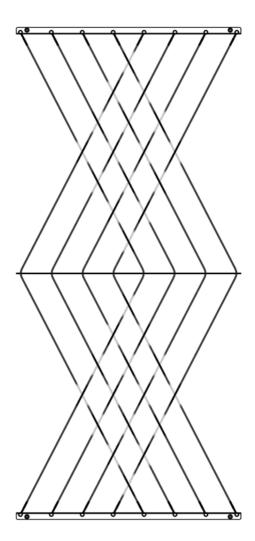
It is recomended to follow the weave pattern as shown above. Wires should be weaved over-under-over-under and so on. Following this pattern will ensure the trellis does not twist. A wire that is weaved over the last wire above the spreader bar should be weaved under the first wire below the spreader bar. A wire that is weaved under the last wire above the spreader bar should be weaved over the first wire below the spreader bar.
